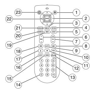
1. () (On/off): Press to turn each monitor/headrest system on or off.
